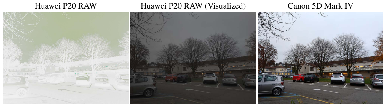
Figure 1. Example images from the collected dataset. From left to right: original 4-channel RAW image (channels = [R, GR, B, GB]) saved in PNG format (transparency channel = GB), original visualized RAW image and Canon 5D Mark IV target image.
