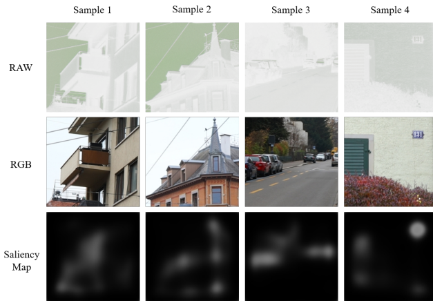
Figure 1. Some training samples. The first row and second row visualize the input RAW files and target RGB photos in ZRR training set. The last row shows the saliency maps generated from the pre-trained SalGAN. For each sample, the training images are paired. Please visit https://github.com/zhaoyuzhi/RAW2RGB-GAN to see more examples and to try our model and code.
