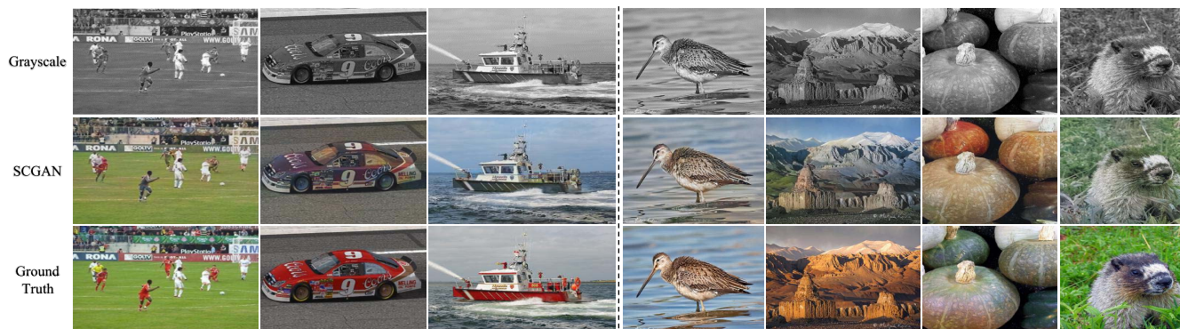
Fig. 14. Examples of the most common failure cases. The top, middle and bottom rows include grayscale ground truth, the generated images, and colorful ground truth, respectively. The SCGAN may be sensitive to small objects like complicated scene, special patterns, and details respectively as shown in left 3 samples. The images generated by SCGAN may be not very colorful, as illustrated in the samples.
