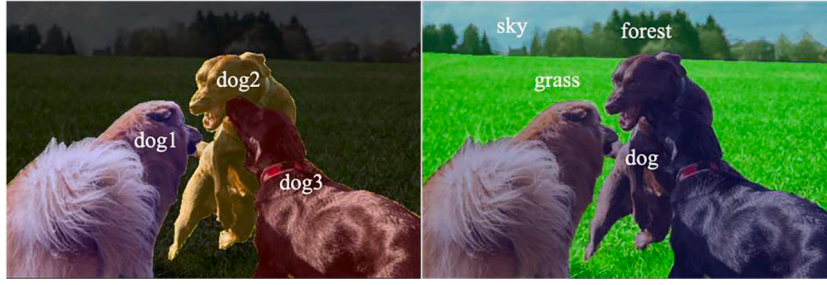
Fig. 1. Comparison of instance segmentation (left) and semantic segmentation (right). Instance segmentation can distinguish different dogs in the same category and labels are only assigned to the pixels within the detected objects. Semantic segmentation can assign a label for every pixel.
